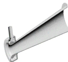
b) Section throughout a Coandă ejector
