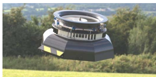
Fig. 16 EMBLA, an emblematic Coandă UAV
