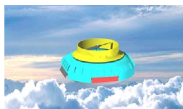
Fig. 17 The Romanian MEDIAS-UAV Coandă effect aerial vehicle meant for environmental surveillance (2009)
