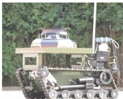
Fig. 17 EMBLA - in its counter IED role on top of a Northrop Grumman Remotec Mk 8 EOD Wheelbarrow
