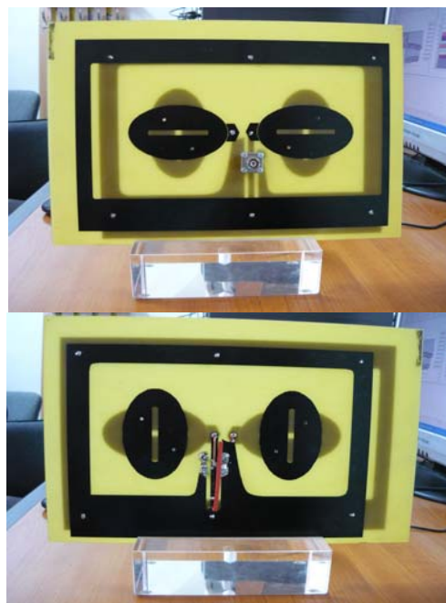
Fig. 14 Front-back view of the stripline antenna with elliptical dipoles
