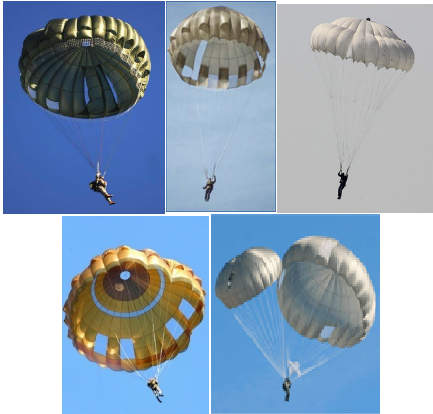
FIG. 2. The round-type parachutes (1-MC-6, 2-GQ 8M-LLP, 3-D10, 4-TAP 696-26, 5- CIMSA TP-2Z)
