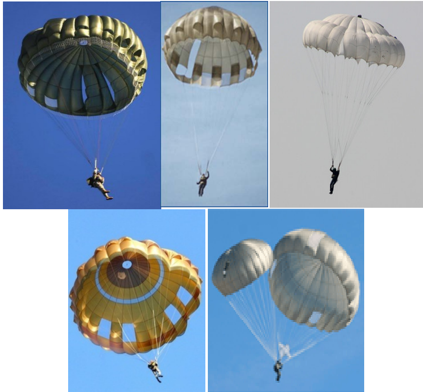
FIG. 2. The round-type parachutes (1-MC-6, 2-GQ 8M-LLP, 3-D10, 4-TAP 696-26, 5- CIMSA TP-2Z)
