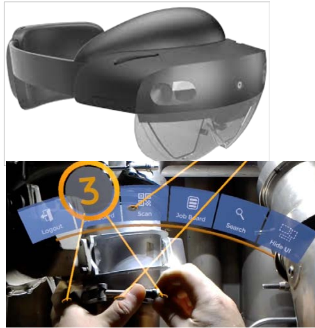
FIG. 2 AR gloves – HoloLens2 (left), capture from op.maintenance using HL2 (right)
