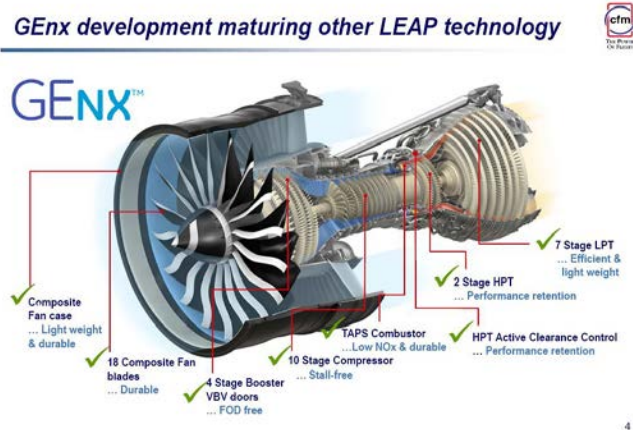
FIG. 14 Design and technology advances in jet engines, GE NX Turbofan Engine, [33]
