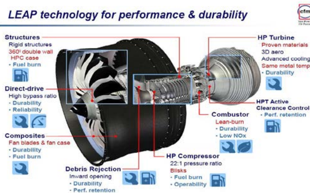
FIG. 15 Advanced LEAP turbofan engines, [34]
