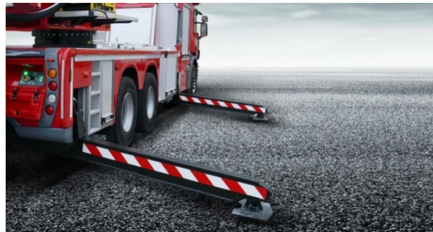
FIG. 9. MAGIRUS M68L escalator mounting system
