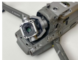
FIG. 30. Drone melted due to excessive heat, [19]
