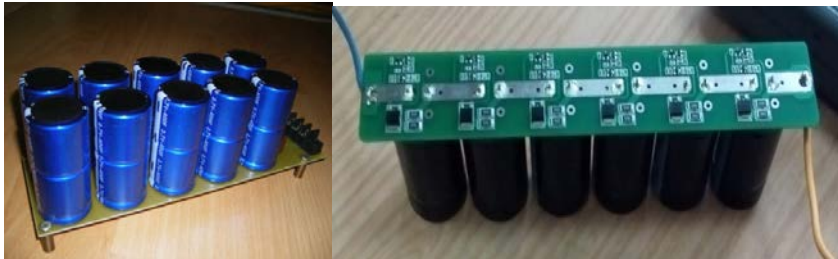
FIG. 3. Super Capacitor Batteries (Heter, left, U_{max} = 13.5 V; GreenCap, right, U_{max} = 16.2 V)
