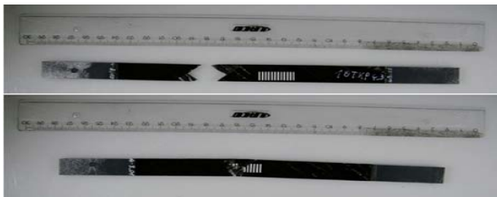
Compression perpendicular on fiber EN ISO 14126
