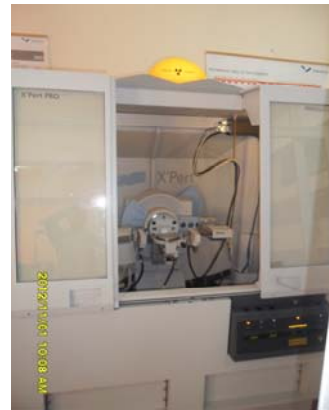
Fig. 2. X'Pert PRO MRD X-ray diffraction installation
