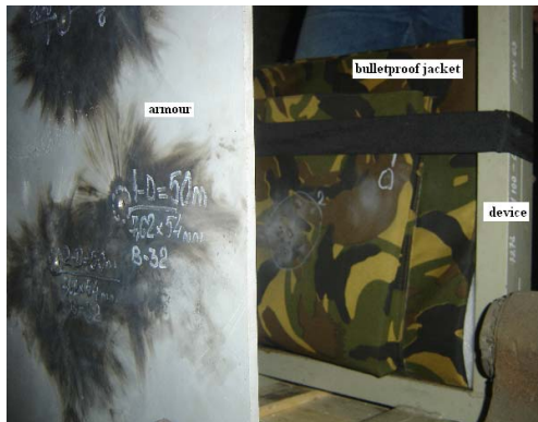
Fig. 2 Impact between 7,62 x 54 mm calibre piercing incendiary bullets and configuration constituted by 6 mm thickness armour plate and bulletproof jacket
