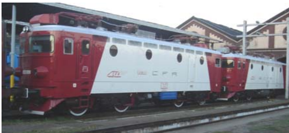
Fig. 3 Electrical railway-engine Bo-Bo type, rehabilitated and modernized
