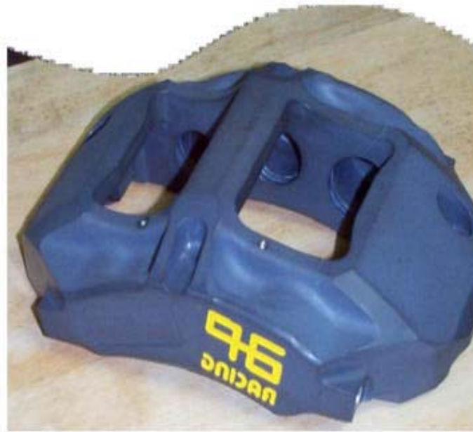
Fig. 3. Example of current production: Brake caliper.
