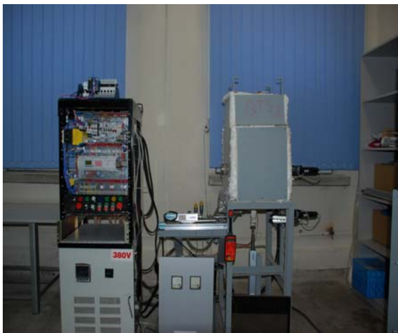
Fig. 3 Quick thermal test shock installation QTS
