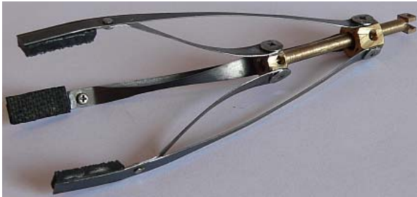
Fig. 11 The compliant minigripper realized
