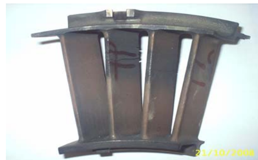
Fig.2 Cracks in the blade's leading and trailing edge because of the thermal fatigue
