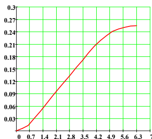
Fig. 1 – Pressure versus time in closed bomb experiments.
