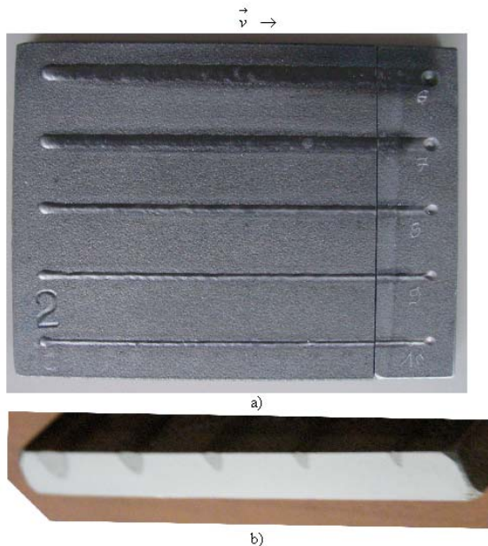
Figure 3 Photograph of the plate 2) Top view b) view section view, from left to right the welds: 6,7,8,9,10
