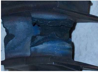
Fig.3 Cracks which lead to tearing of the material
