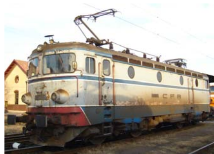
Fig. 2 Electrical railway-engine type Bo-Bo of 3400Kw
