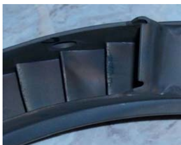
Fig.1. Corrosion stains and asperities on the stator blades
