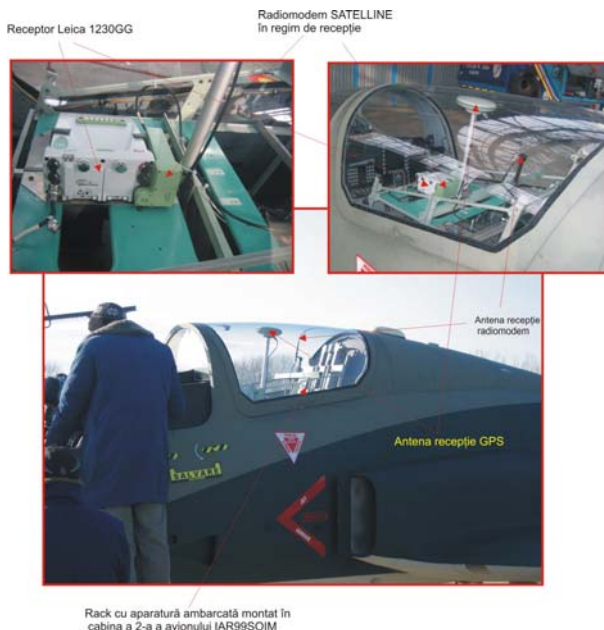
Fig. 3. The solution of instrumentation with DGPS/RTK on IAR99SOIM aircraft
