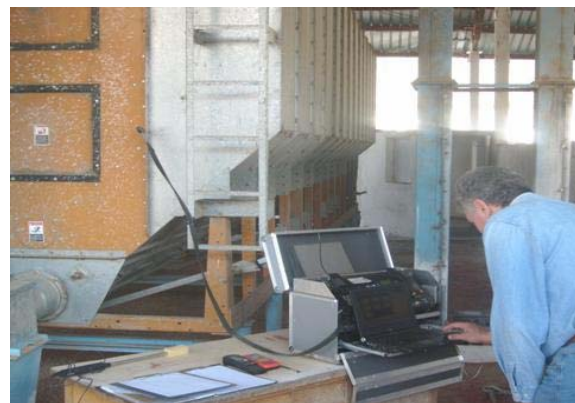
Fig 6 Pollutant emission acquisition form the flue gas during corn drying process
