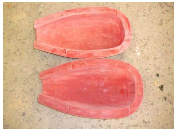
Fig.2 NOTAR- body of carbon fiber
