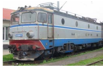
Fig. 1 Electrical railway-engine type Co-Co of 5100Kw
