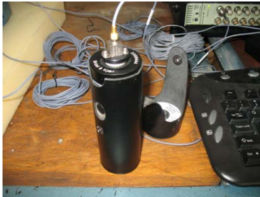
Fig. 3 Calibrator type 4294 with transducer of 4508 B 001 type
