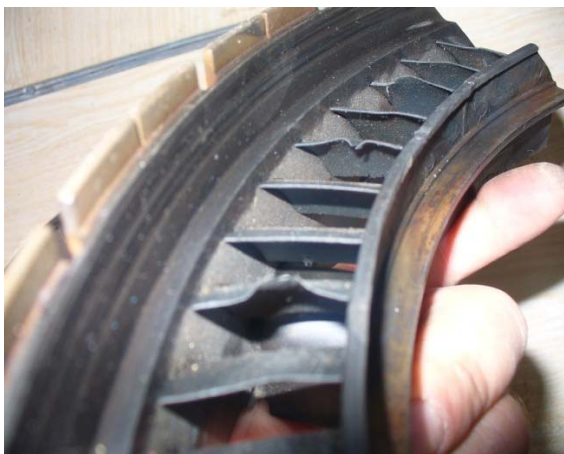
Fig. 5 Superficial disruption of the turbine's stator blades
