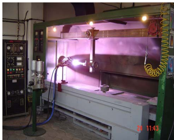
Fig. 2 Samples realization - APS technique
