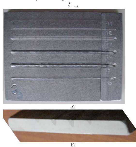
Figure 4 Photograph of the plate 3) Top view b) view section view, from left to right the welds: 11,12,13,14,15,36
