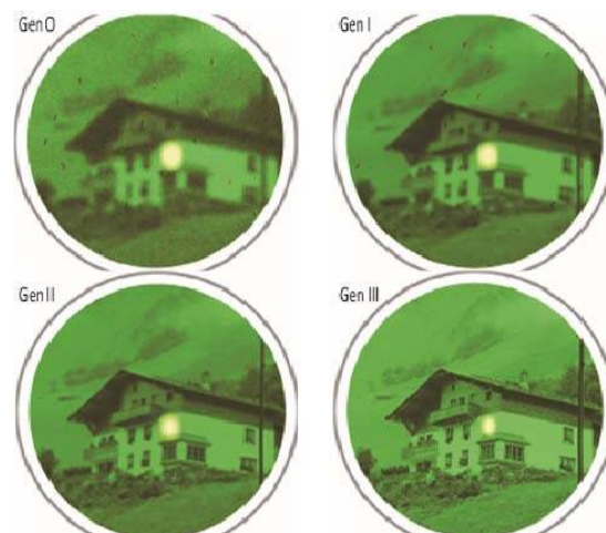
FIG. 1. Technical generations of night-vision optoelectronic systems with image intensifiers
