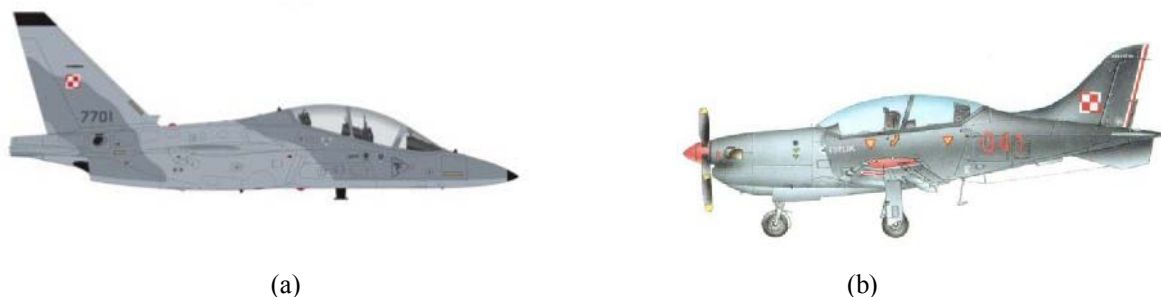
FIG. 4. (a) M-346 Master - military twin-engine transonic trainer aircraft, (b) PZL-130 Orlik - Polish turboprop, single engine, two seat trainer.
