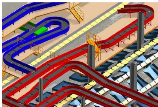
FIG.3. Hold- Baggage System
