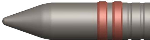
FIG. 5. Projectile 30x210B for NN-30 canon 3D virtual model, configuration 4-30 (Source: Authors database presented in [1])
