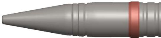
FIG. 4. Projectile 30x165 for Gsh-30 canon 3D virtual model, configuration 3-30 (Source: Authors database presented in [1])
