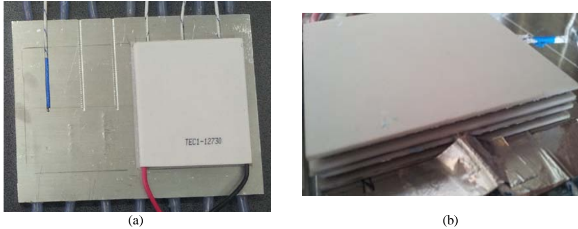
FIG. 3. The thermoelectric generator's (a) cold part connected with aluminum block (b) hot part connected with other thermoelectric device
