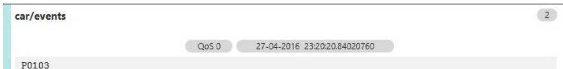
FIG. 9. Mosquitto broker receiving P0103 error code form Moquitto client over the IP network.
