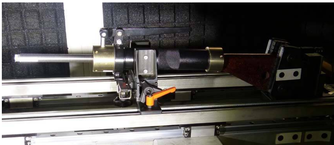
FIG. 6 Mechanical recoil setup on the firing rest
