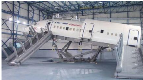
FIG.3.1 Electrically driven platform of a flight simulator Source: www.boschrexroth.com
