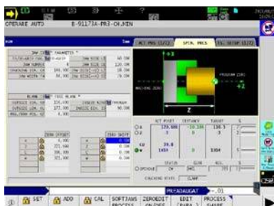
FIG. 19. MDI mode of Okuma CNC machine
