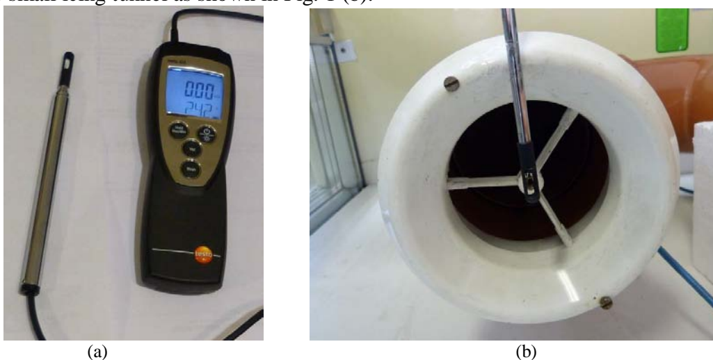
FIG. 1. Thermal anemometer Testo 425 (a), hot-wire probe attached in test section (b)
