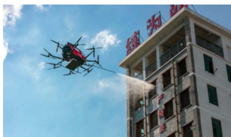
FIG. 26. EHang 216F drone intervention scenario at a tall building
