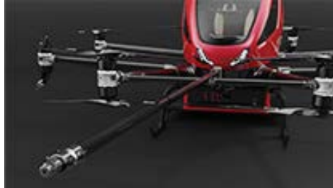
FIG. 28. EHang 216F drone extinguishing hose
