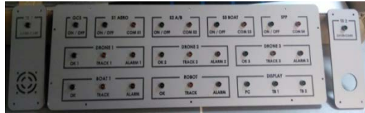
FIG. 3.4 Realization of the upper signaling panel through CNC technology
