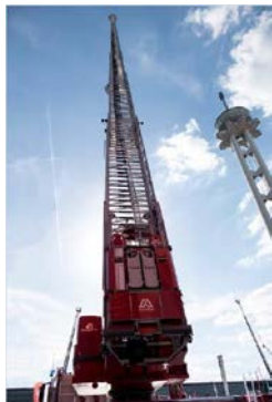
FIG. 8. Lifting and stretching the ladder package of the MAGIRUS M68L escalator
