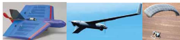
Fig.1 Robotic aerial systems - Flying wing type. a. EADS, Germany (plank) b. EagleScan, USA (swept) c. Snowgoose, Canada (parafoil)
