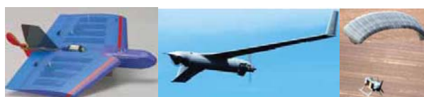
Fig.1 Robotic aerial systems - Flying wing type. a. EADS, Germany (plank) b. EagleScan, USA (swept) c. Snowgoose, Canada (parafoil)
