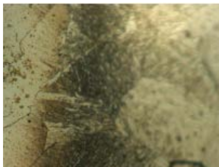
FIG. 5. Sample 5 - heating to 1100 °C for 30 minutes and cooling in water, followed by tempering at 500 °C for 30 minutes and cooling in air. Aqua regia etching. 500:1
