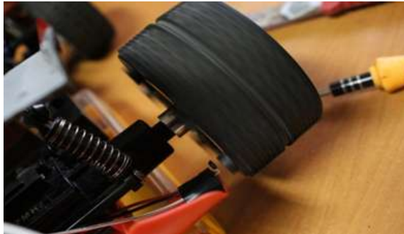
FIG. 8. Hall sensor and/with magnets on the engine wheel – test
