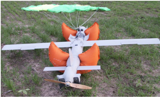
a. Recoverable parachute and airbag [4]
