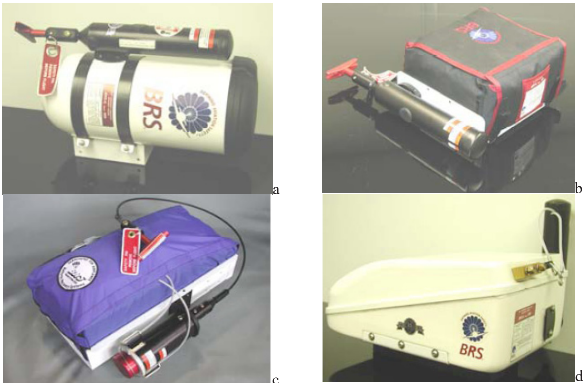
Fig. 2.5 BRS rescue and recover systems [14]
