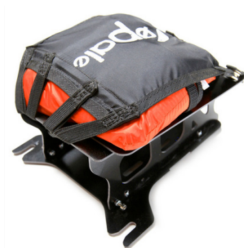
Fig. 2.2 Multi-rotor recover kit and recovery parachute [10]
