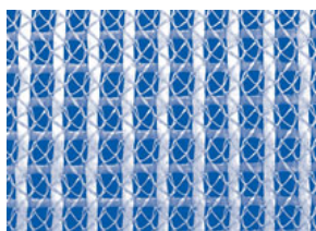
Figure 2. Illustration of a stitch-bonded fabric
