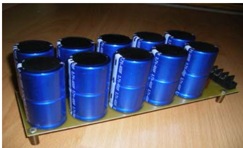
Fig. 1. Example of supercapacitor battery (2x400/5F, 13.5V)
