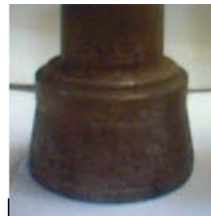
Fig. 4: Punch loaded by welding
