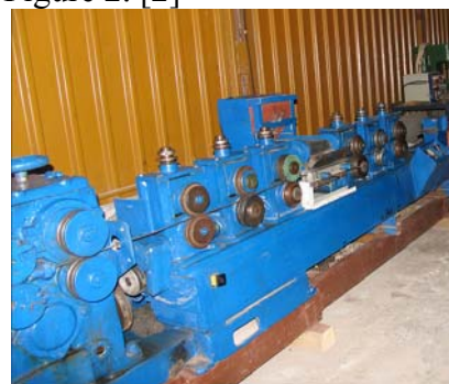
Fig. 2: Tubular rods production line
