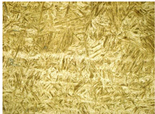
Fig. 5 Microstructure of HAZ (area close to weld metal), 500x
