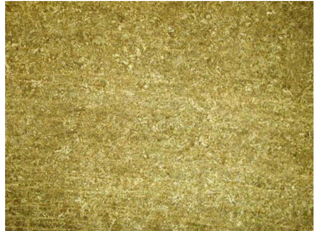
Fig. 4 Microstructure of base material (ARMOX 500), 500x
